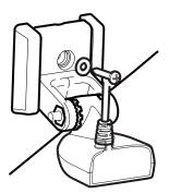
4. Snap the pivot back down. Install #8 x 1" wood screw into the 4th hole to lock down the pivot arm. Hand-tighten only!
